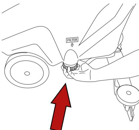
Check that the detergent outlet filter is clean.
