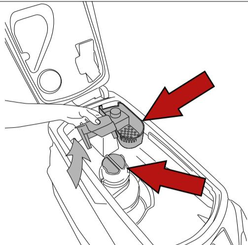
Check that the suction filter and dirt filter are clean.
