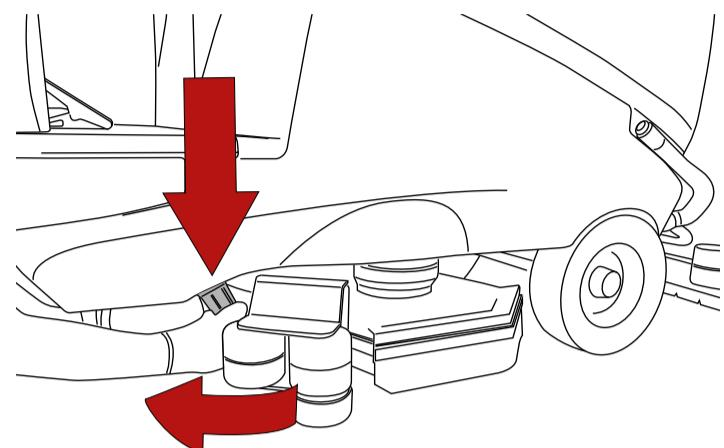
Check that the detergent outlet filter is clean.
