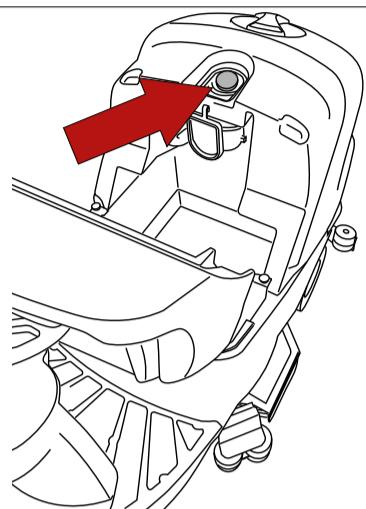
Check the suction filter is undamaged and clean.
